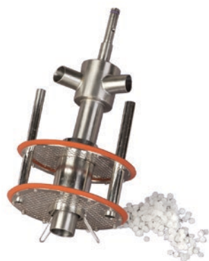
Figure 2: Packed-bed basket with Fibra-Cel disks
