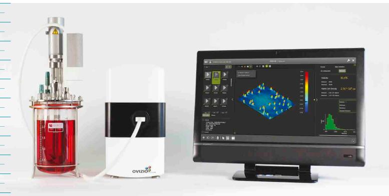
The iLine Fast is connected to bioreactors via a specific, sterile closed loop disposable fluidics system. Cells are pumped out of the bioreactor, via an innovative pumping system, flow through the imaging device in a temperature-controlled environment and flow back to the bioreactor after the holograms of the cells have been captured. The holograms are continuously analyzed to compute cell density and cell viability.
