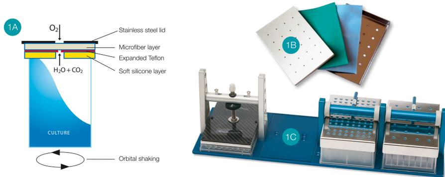
Figure 1A | Representative well of a microtiter plate, covered with a layered lid-system comprising of stainless steel, microfiber, expanded teflon, and soft silicone. Some of the layers are perforated to allow for adequate gas exchange whilst maintaining sterility.
